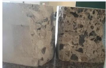
Figure 3.28. Typical crack under 4-PBT using 100x100x300 mm specimen
