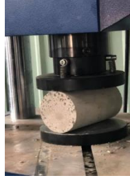
Figure 3.6. Splitting tensile strength test
