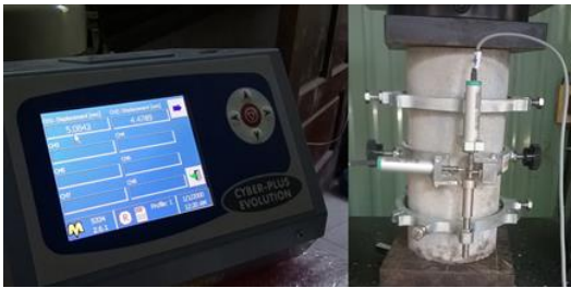
Figure 3.5. Test for Static Modulus of Elasticity and Poisson's Ratio
