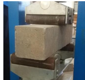
Figure 3.7. Test for flexural strength- 4 point bend.
