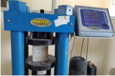
Figure 3.2. Compressive strength test
