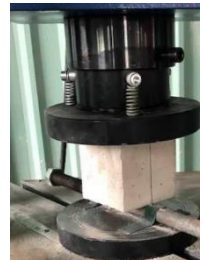
Figure 3.6. Splitting tensile strength test
