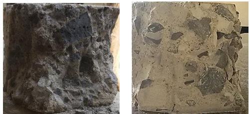
Figure 3.8. Failure surface of steel slag and natural concrete
