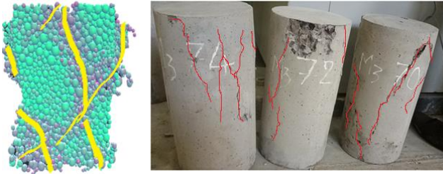
Figure. 5.11. The cracks in the numerical sample and experimental specimens
